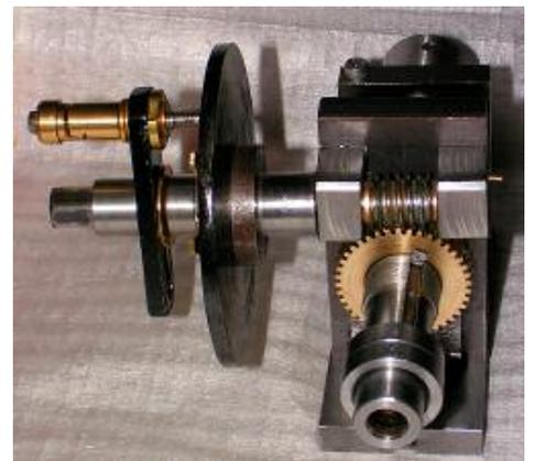
The spindle was case hardened so I used a carbide tipped tool to turn down the spindle nose and cut the thread. After I cut through the hard surface the material machined very well.
